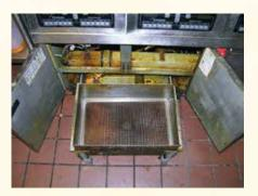
Open the fryer doors and pull the filter pan out. Remove weight ring, but leave the screen in place at the bottom of the well.
