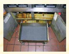
Insert the F-54 CarbonPad into the pan with the bumpy side up. The CarbonPad will fit "edge to edge."
