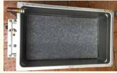
Before assembling the filter pan unit, be sure to clean and dry any water in the pan. Place the support screen in the center of the pan.
