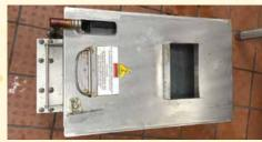
Henny Penny Evolution Elite requires several oil filterings throughout the day in all fry vats. WHEN NEEDED, scrape the crumb debris off the CarbonPad before continuing the oil filtrations. Please allow filter pan to cool before scraping CarbonPad. Removing crumb debris will help oil flow back to the fryer vats. Use one CarbonPad and replace at start of each day.
